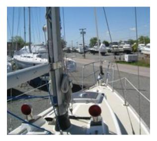
The aluminum mast (with internal furler), boom, and related winches and hardware are in good serviceable condition, as can be inspected from on deck. The spreaders are in good condition. The shrouds, and turnbuckles also check out fine. The mast step is well secured, and the mast step shows no signs of corrosion. The step is properly fitted to the keel. All deck hardware, including winches, is properly backed.
