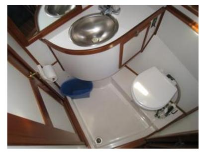
Both forward and aft heads are good sized and equipped with showers and manual marine toilets that discharges into bladder type holding tanks, or can be pumped overboard via a proper Y-gate. There are hand wash basins in both heads and a fiberglass tub installed aft. No wood rot was noted in these areas. The heads are finished in Teak and Mahogany and are exceptionally clean. (Aft head Photos on Page 6).
