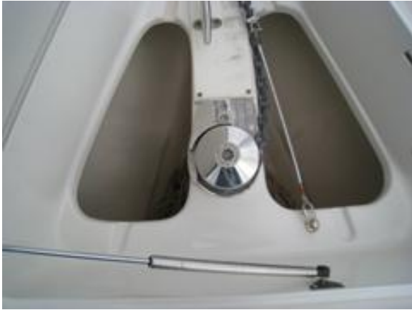
Windlass mounted in anchor locker
